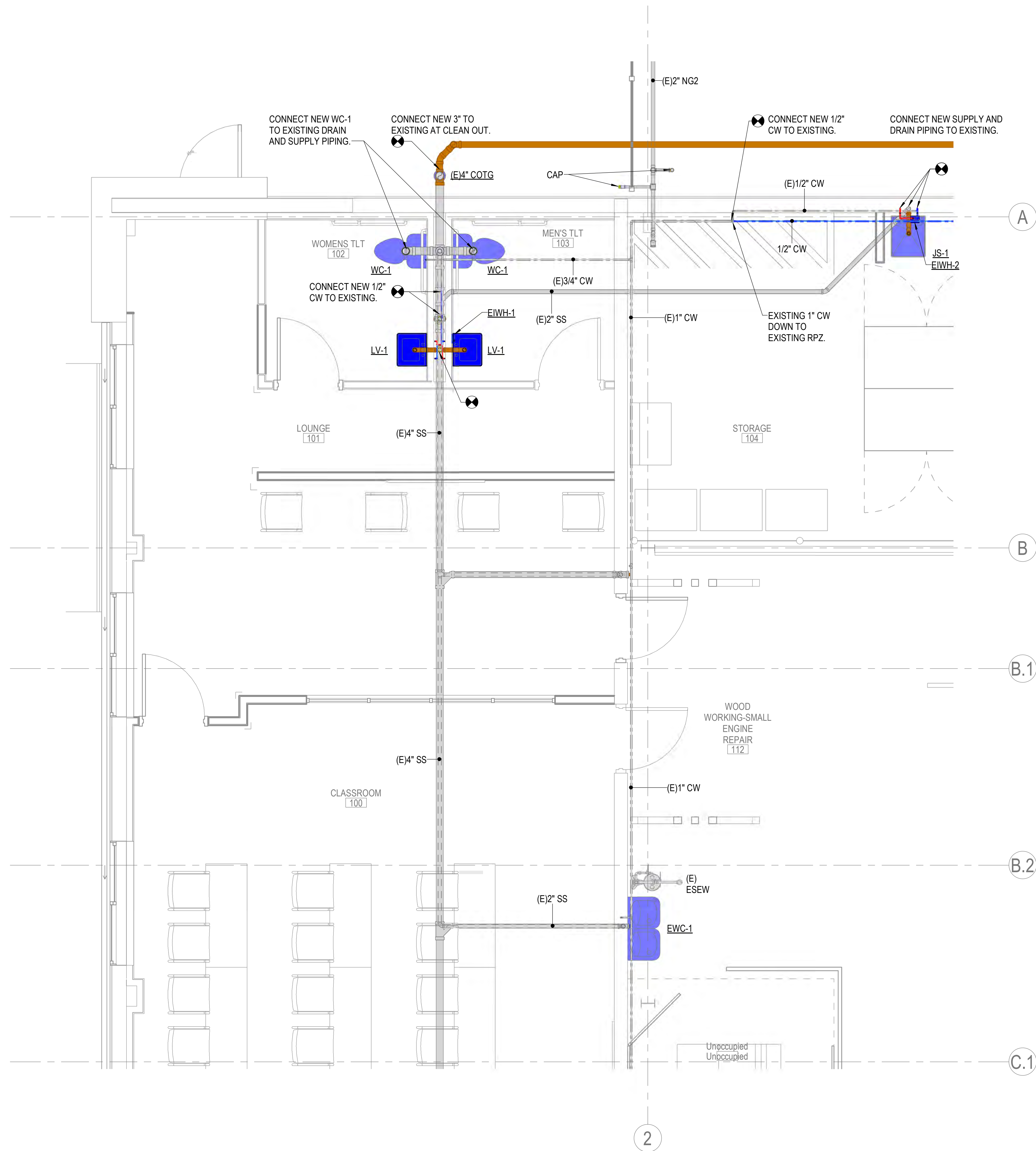
1 ENLARGED FIRST FLOOR PLUMBING PLAN - WEST RESTROOM 3/8" = 1'-0"
